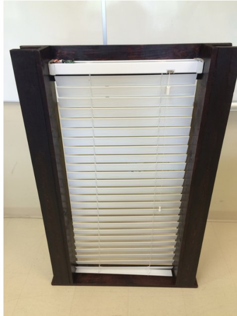
Figure 1. Blinds Frame Setup (Backside/Indoors)
